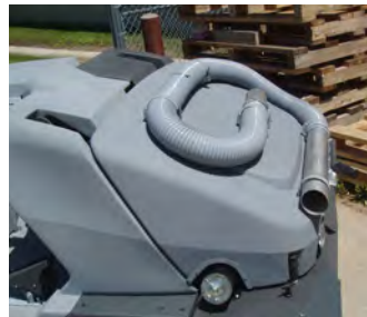
Litter vac Suitable for cleaning hard to reach spots like dock plates, under steps or shelving etc.
