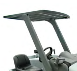
Overhead guard For additional operator safety, especially in warehouses and industry
