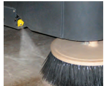
DustGuard™ kit To control air borne dust on the side broom/s
