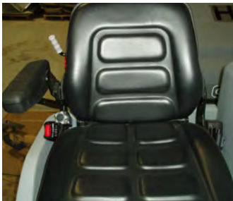
Suspension seat Comfortable seat with adjustable suspension based on operator's weight
