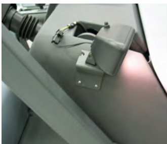
Working light front The front and rear lights provide light on focused areas where the headlights do not reach
